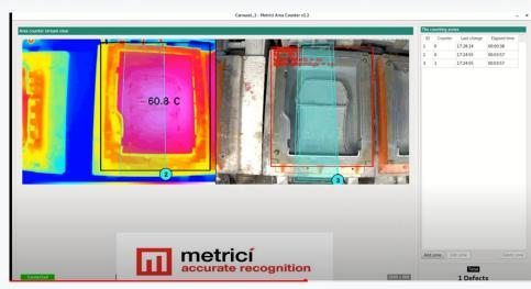
Metrici instructs the robotic arm to not pour the foam into the mold – as a defect would result
